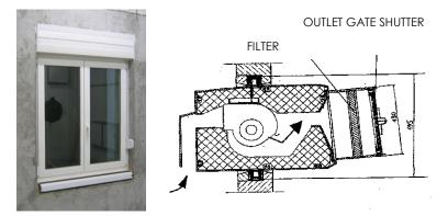
Figure 12: Auto-ventilating window (on the left, the aerator is located in the lowest part of the window) and section of the aerator (on the right)
