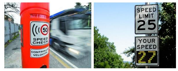
Figure 16: different types of speed reduction devices: speed checker (on the left) and radar speed sign (on the right)
